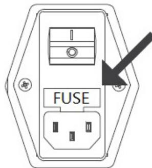
**Fig. 44 - Fuse compartment**
